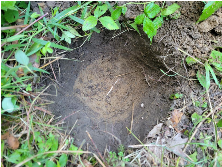
Image 10: Open Test Pit showing Subsurface Stratigraphy.
